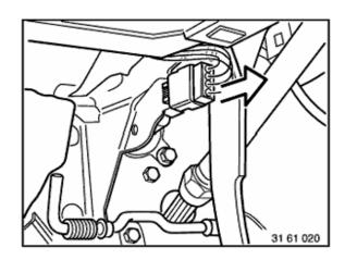
Removing instrument panelling at bottom left, refer to 61 31 016
